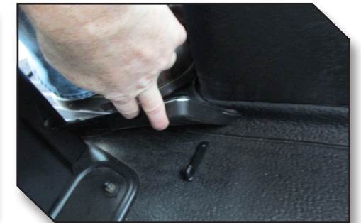
Figure 12 – Properly Installed Hook
