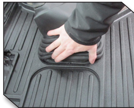
Figure 6 - Straightening Rubber Boot
