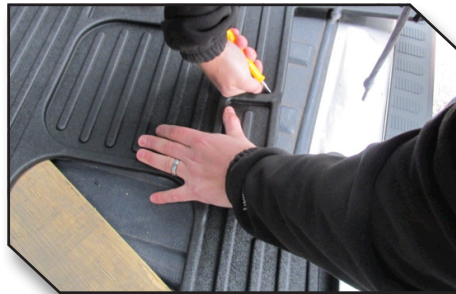
Figure 4 – Trimming With Utility Knife
