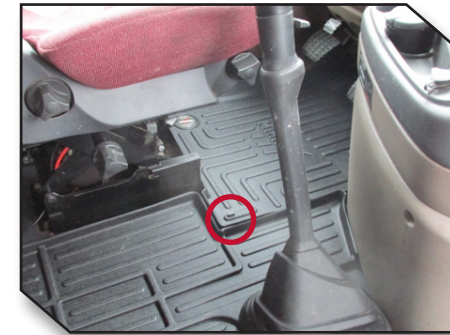
Figure 10 – Confirm Location Driver Mat and Hook
